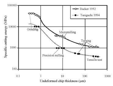
Figure 1: Variation in specific cutting energy for three major machining processes [16].
