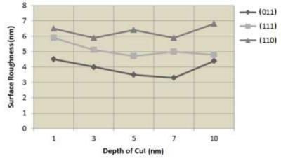
**Figure 2:** Effects of the crystallographic orientation and the depth of cut on the surface roughness conducted by the diamond turning of single-crystal aluminium roods [15].
