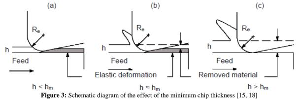
In figure 3 (a) the uncut chip thickness (h) is less than the minimum chip thickness (hm). The cutter (edge radius Re) deforms elastically the workpiece and no chip is formed, chips formed in a discontinuous way
